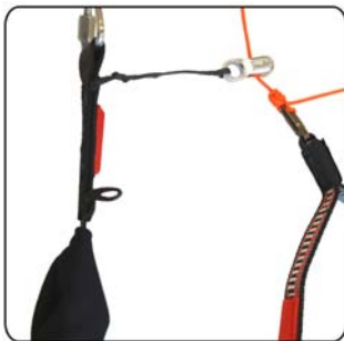
Upper position of brake guide pulley
