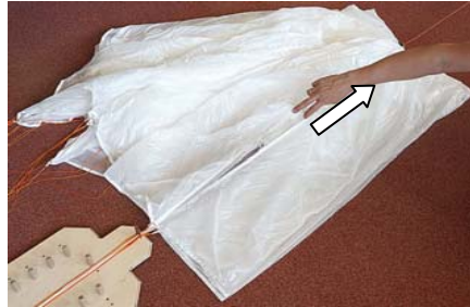
11) Pull the upper edge of the corner slot towards the top of the canopy to stretch the corner line.
