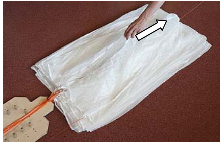
28) Pull the upper edge of the corner slot towards the top of the canopy to stretch the corner line.
