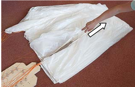
16) Pull the upper edge of the corner slot towards the top of the canopy to stretch the corner line.
