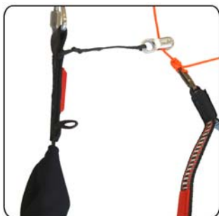
Upper position of brake guide pulley
