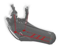
Test your speed system for the correct length of cord on the ground first (simulating flying position), with your harness and risers, before flying with it! The full range is reached when the 2 pulleys join together.
