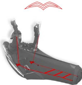
Test your speed system for the correct length of cord on the ground first (simulating flying position), with your harness and risers, before flying with it! The full range is reached when the 2 pulleys join together.
