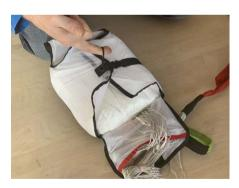
Lead the black rubber loop trough the grommet of the leaf no. 2.
