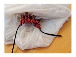
The packing line for holding the packing loops together can be removed now. It is important that this line is removed completely. Otherwise it will prevent the opening of the Aegis SQ!
