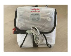
Use the remaining free line to secure the black rubber loop of the inner container.
