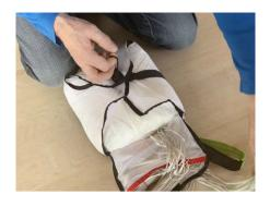
Lead the black rubber loop trough the grommet of the leaf no. 3.
