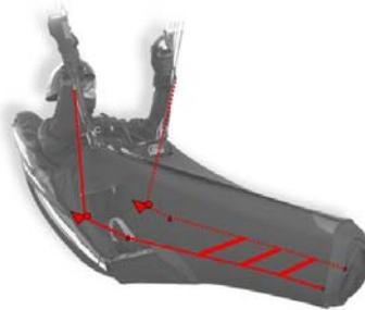
Test your speed system for the correct length of cord on the ground first (simulating flying position), with your harness and risers, before flying with it! The full range is reached when the 2 pulleys join together.
