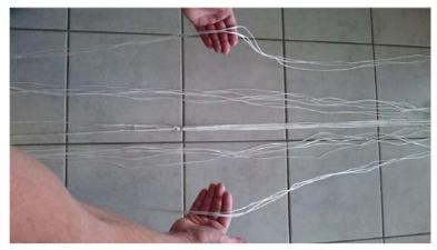
Follow the brake lines from the brake line riser to the canopy and check for twists.
