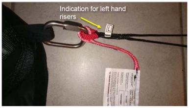
Install only approved connectors with at least 250 kg WLL (Work Limit Load). If you use Dyneema links, install them according to the instructions of the manufacturer. **Put both loops (riser and red safety connection) on each side into the shackle and tighten!** If your harness has an included V-line, remove it.
