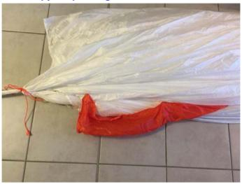
Bundle the lines with a packing rope and fold the right side of the canopy over the left side, so that the red marking of the front tip, that shows the flight direction, is closed to you.
