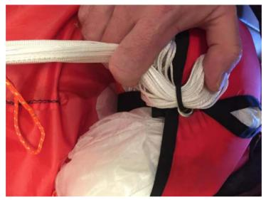
Take the rubber loop and both leaves of the container and close it with the bundle of lines. Only lead the rubber loop through the two lugs.
