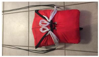
The redundant loops to close the container prevent an inadvertent or too early opening during the extraction of the container from the harness.
