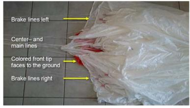
Front tip and harness faces in flight direction to the ground.
