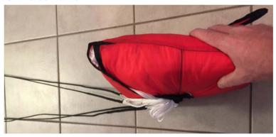
Twist the container  $180^{\circ}$  counterclockwise (direction of rotation, if you look in direction of the harness) and if the reserve parachute will be installed on the right side of the harness. Otherwise opposite.
