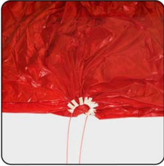
1. Slide on the packing-loops on a line (packing-cord), and hook it in.
