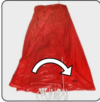
2. Segment 9 (Aegis 30), Segment 12 (Aegis 33 and Aegis 38), Segment 10 (Aegis 63) have to be put on the right side
