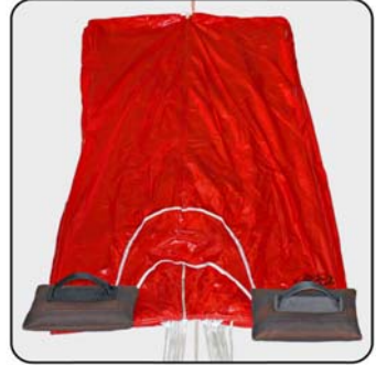
6. Check that all lines and the center line are not crossed and running free.
