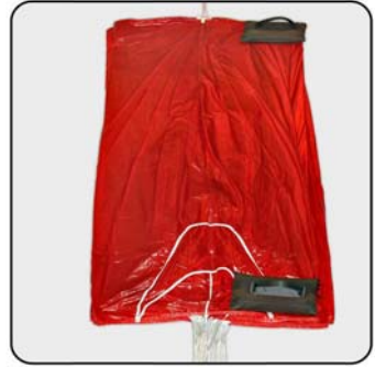
3. Lay all segments until segment 1 (stamped segment) is on the top, then put a weight (sand bag) on it.
